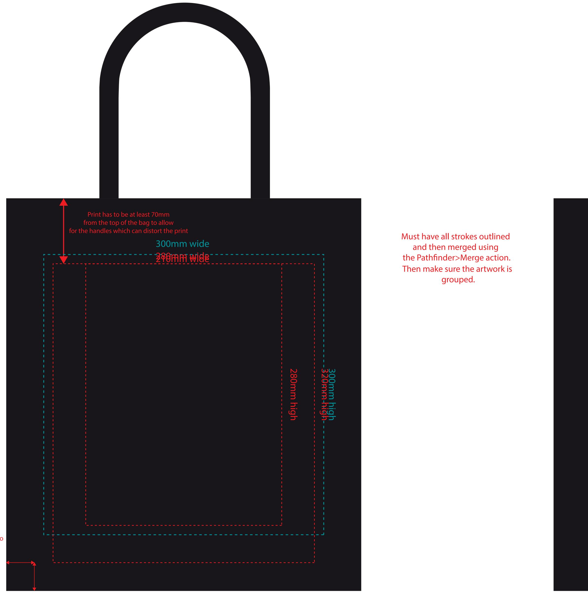
The closest we can print to the edge and bottom of the bag is 30mm.
