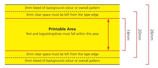
**Printable area:** This area is 3mm inside the top and bottom edge of the tape, giving a printable area of **14mm** high. Logos and text must fall within this area to ensure no clipping occurs.
