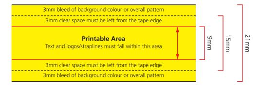
**Printable area:** This area is **3mm** inside the top and bottom edge of the tape, giving a printable area of **9mm** high. Logos and text must fall within this area to ensure no clipping occurs.
